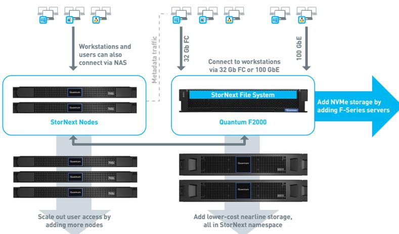
With the F-Series in a StorNext shared storage environment, users access data directly from the storage—either on the SAN or on an IP network—without the bottlenecks associated with current storage and networking technologies. The result? Dramatically lower, and predictable, latencies for anyone working in UHD and high-frame-rate content.
