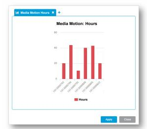
This report example shows drive usage (tape motion hours) for six drives in a partition. This graph suggests that reallocating jobs to underutilized drives could better balance the drive workload.
