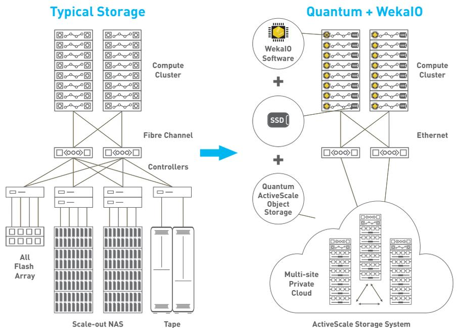
Figure 1: The Quantum+WekaIO solution combines the performance of flash with the durability and efficiency of object storage.
