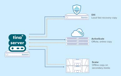
Example 3-2-1-1 Solution for Enterprise Deployment. Applying the 3-2-1-1 best practice for a scalable enterprise deployment might include an Enterprise media server based on Atempo Tina, a local DXi appliance for high-speed backup and instant recovery, an ActiveScale object store deployed offsite as S3-compatible private cloud storage, and a Scalar tape library for offline copies written to secondary media.
