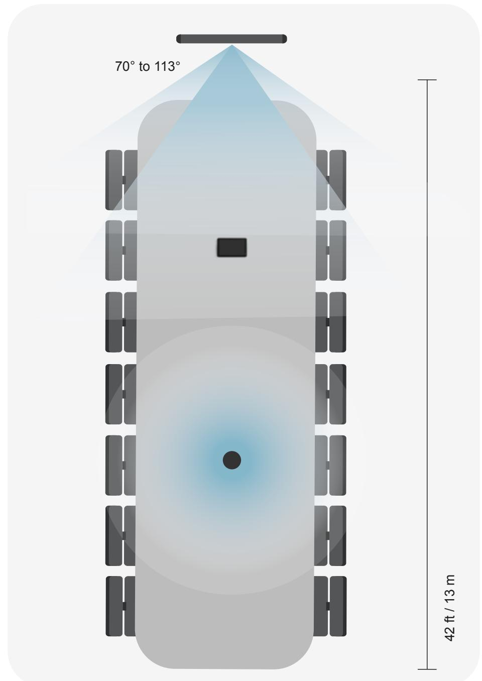
Neat Center provides an additional 15 ft of microphone and camera coverage from where it is placed. Meeting experience will vary based on placement of Neat Center.
